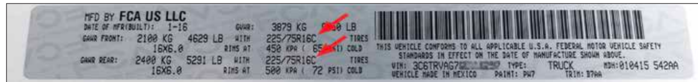
FIGURE 1 (Above): Example Vehicle Certification Label
