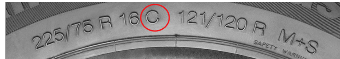
FIGURE 3: Size and service description of an example C-Type European Commercial Metric Tire
