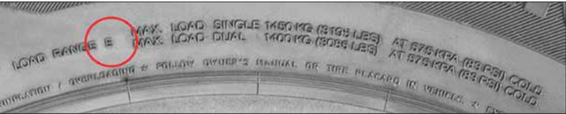
FIGURE 4: Load range, max load and pressure specifications for the example tire shown in Figure 3
